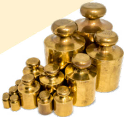
A set of weights used on the balance machine at the Royal Mint Refinery to give an accurate account of the weight of gold received
