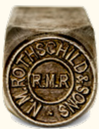
The stamp used to imprint Rothschild & Co identification marks onto products (primarily gold bars) of the Royal Mint Refinery'
